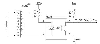
Here is how Inputs are connected. You can see input switch and one of 4 9-wire BRK terminals on the left. The topmost terminal is Machine-Side signal ground. SVcc is Machine-Side +5V power. They are connected to the BRK +5V power supply on the BRK. It is easy to see that current will flow from SVcc through R\_LED and optocoupler LED to SGND if switch is closed. That current will lit the LED. Light emitted by the LED will make the transistor to
