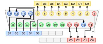
This is how PC parallel port looks to the outside world and to the software that works with it. As you can see there are 4 groups of pins in a single parallel
