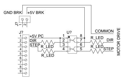
Top connector here is BRK topmost right 2-pin terminal providing *Machine-Side* +5V power. Dual optocoupler shown on the schematic but any single, dual, or quad optocouplers can be used here. It is better to use ones with 100% CTR (Current Transfer Ratio) but anything will work if motor drive's input optocouplers are sensitive enough (2.5mA or so.) Gecko's G203V are. Left pair
